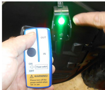
8. Slide Wireless Remote Up to the On Position. Press Upper Button.
