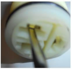
2. Insert thin release blade to unlock wire connector.
