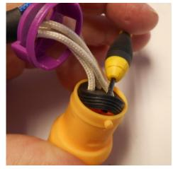
1. Unplug and remove rubber plug, slide back.
