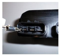
4. Install all 3 wire clips in any order to the 3 male spades in the Regulator/Rectifier.
