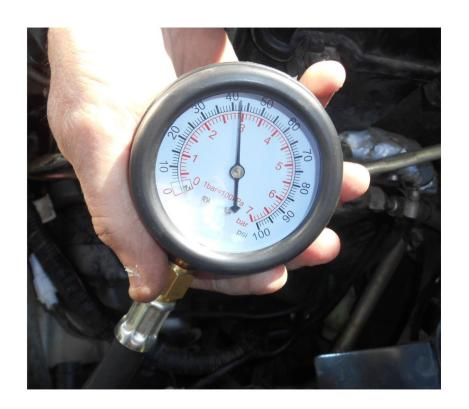
With just "Key On' the pump will cycle up for 3 seconds. The ECU turns off the Ground Negative 12v., until the engine is started.
