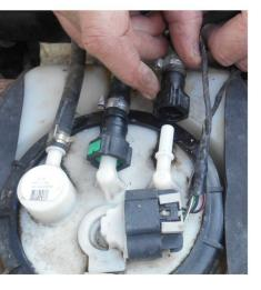
Remove 'Return' fuel line from pump by compressing both locking tabs.
