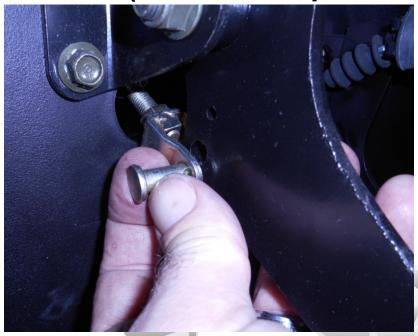
The Brake Foot Pedal must have a small amount of freeplay, approx 1/4". This allows the master cylinder plunger to return to its full closed position.
