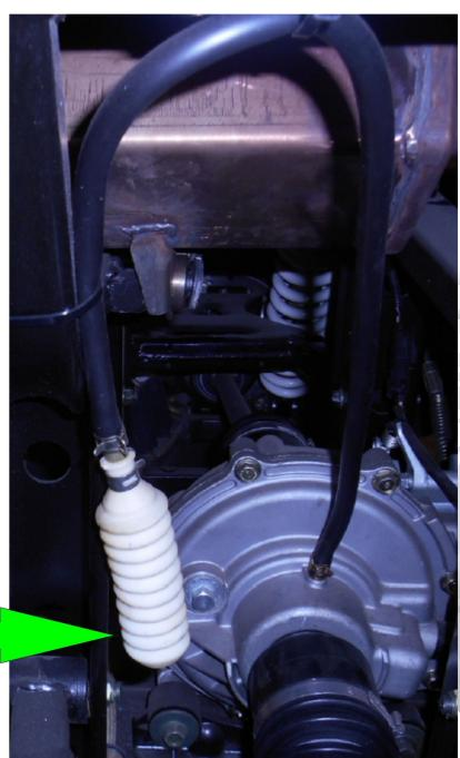
This is found on the Hs1000 rear differential. This air tight flex boot should be added to ALL HiSun UTVs and ATVs, Front and Rear!
