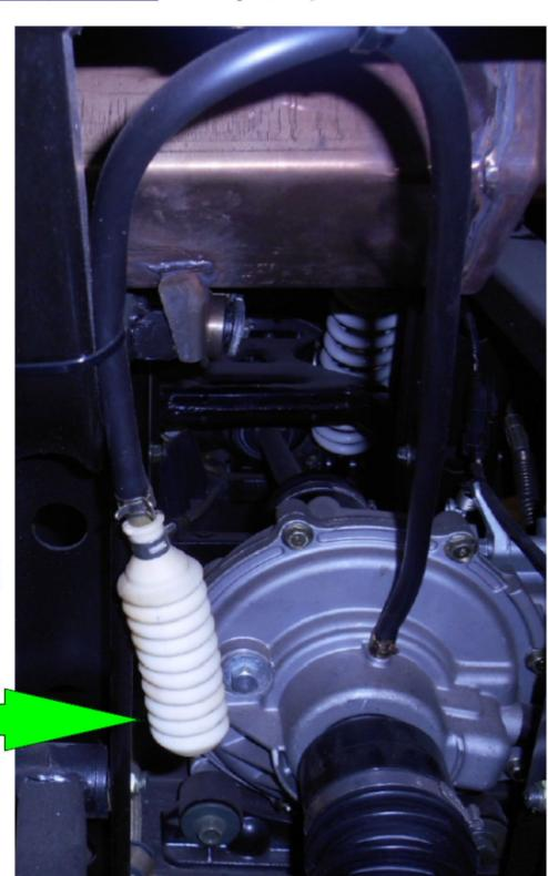
This is found on the Hs1000 rear differential. This air tight flex boot should be added to ALL HiSun UTVs and ATVs, Front and Rear!
