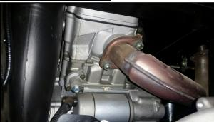
8. Remove [2] 13mm exhaust flange nuts and remove header.
