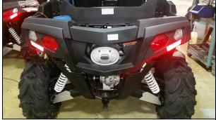
Remove the [4] exhaust spring that hold muffler to mid-pipe, remove the [2] 10mm.bolts from muffler mount and remove.
