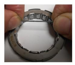
Cut off approx. 15mm, push and twist together, install.
